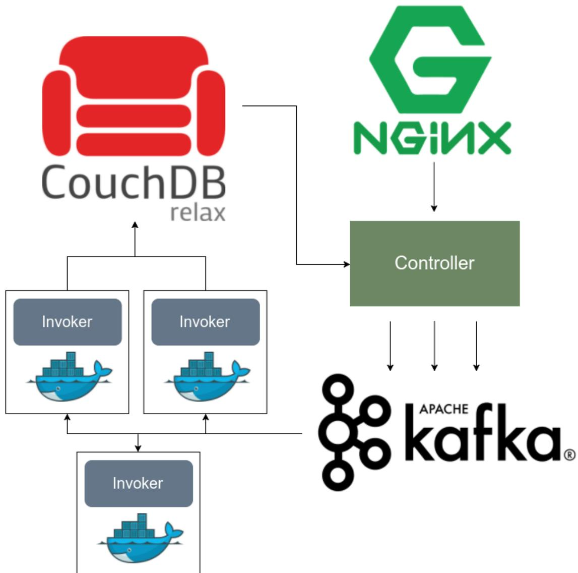
Figure 152: OpenWhisk workflow
