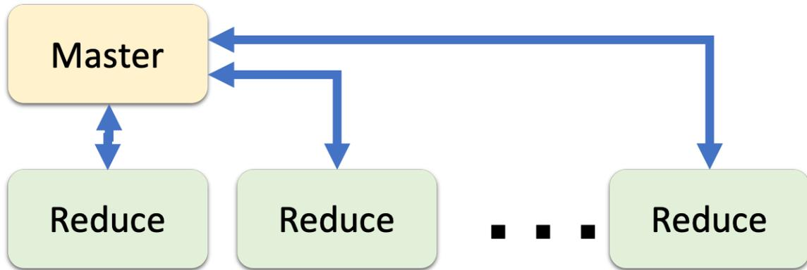
Figure 92: MapReduce Master worker diagram
