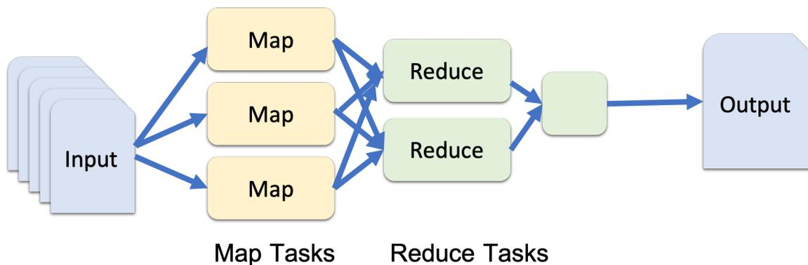
Figure 91: MapReduce Conceptual diagram
