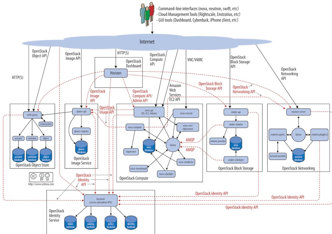
Figure 90: OpenStack Architecture
