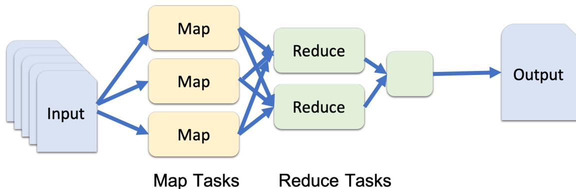
Figure 91: MapReduce Conceptual diagram
