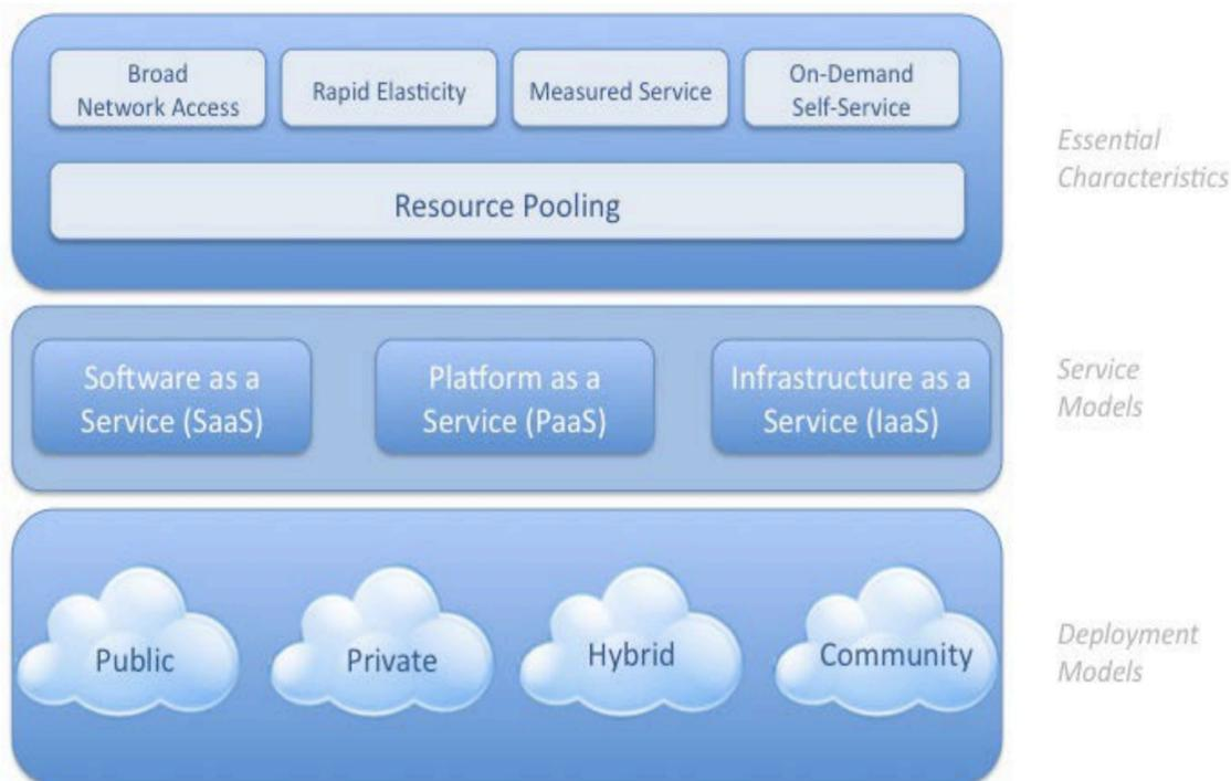
Figure 30: Visual representation of the NIST Cloud Architecture [Source](#)
