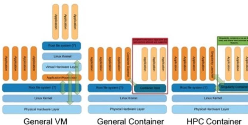
Figure 139: Singularity Container Architecture [97]
